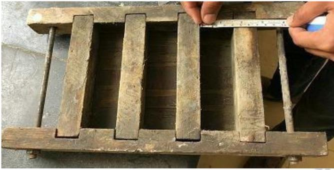
**Fig 2: Moulds for Prisms of Size 40mm\*40mm\*160mm.**
