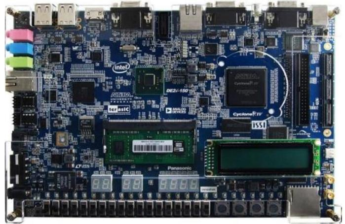
Fig.10: FPGA hardware platform set-up
