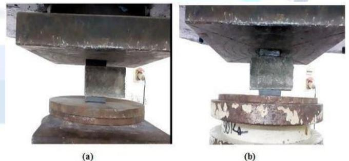
**Fig 5: Different Arrangements of Bearing Plates on UTM**
