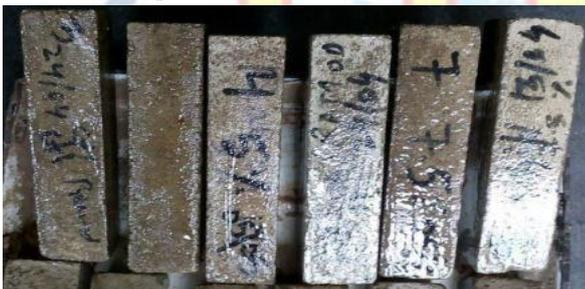
**Fig 3: Prisms with Epoxy Coating**
