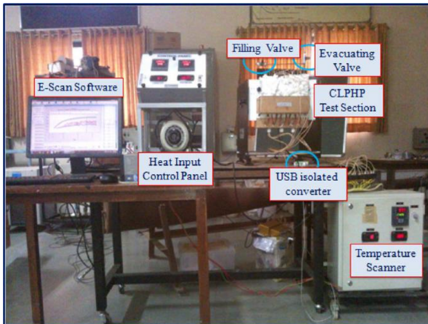
Fig. 3. Experimental set up for a CLPHP. [1]
